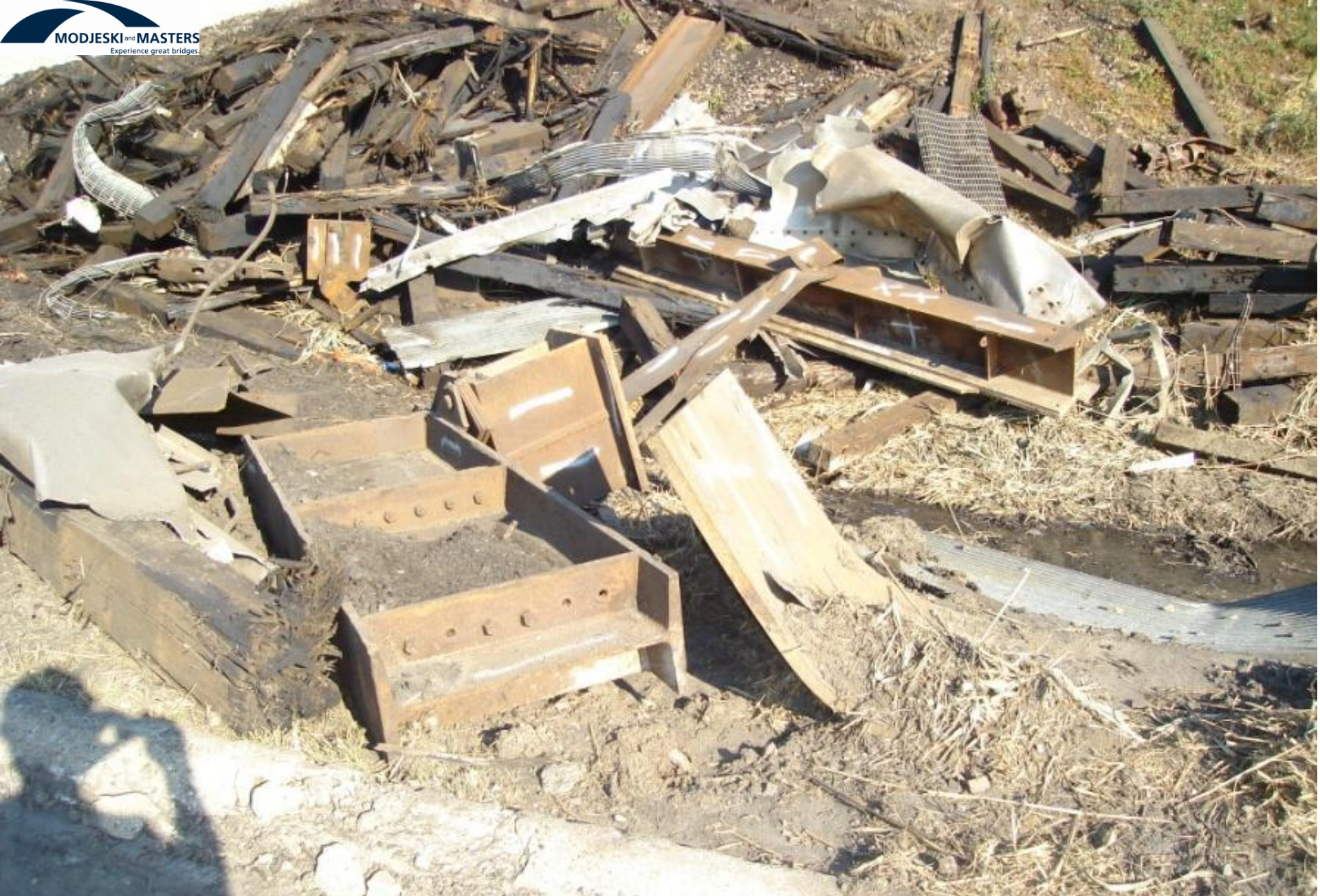
View of multiple bridge components all in full section and good condition. Left center – 9 ' long beam (jump span) Far center - grillage assembly
