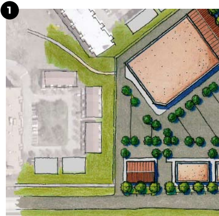
Pedestrian connections to adjacent neighborhoods should be created wherever possible, such as this one from Central Road to the Dearlove triangle.
