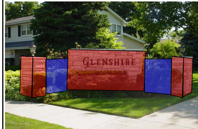
The three elements together (monument & 2 pillars) equal more than 60 cubic feet. The fence is compliant, but the 2 pillars would most likely have to be removed to meet the design guidelines (-103 cu ft) (2.5)
